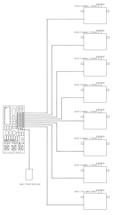
Make sure the + and – polarity of your servo cable matches the pins on the module
